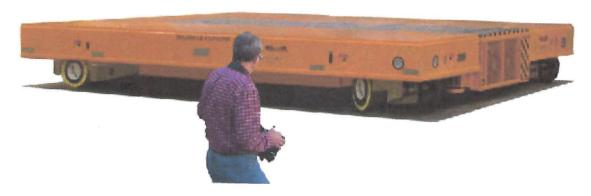
Offering 100 ton capacity, Self-Propelled Trailer features SynchroSteer® computerized independent steering, Uniload® on-center rotating front axles, remote control operation, and on-board power generation. Unit measures 21 x 8 ft with 27 in. deck height and 15 x 7.5 in. solid urethane wheels that operate on any floor surface. With recommended speeds from 0-100 fpm empty and 0-70 ft loaded, trailer is suited for in-plant operation in congested, confined areas and narrow intersecting aisles.
