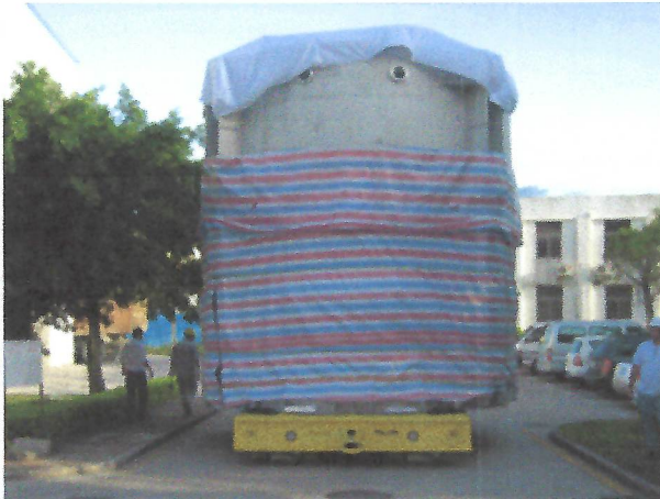
Figure 2: Wheelift heavy transporters are available that are capable of lifting up to 150 tons each.
